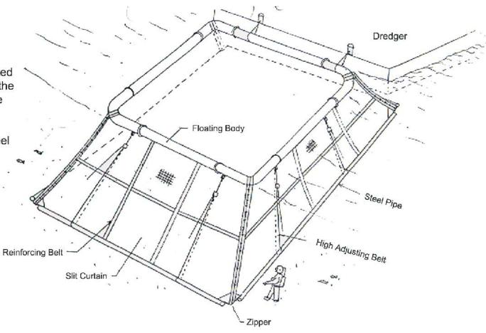
DESIGN OF THE SILT CURTAIN FOR TUEN MUN UNDERWATER TRENCHING AS DESCRIBED IN EP CONDITION 2.3
